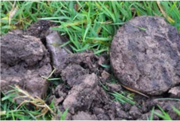
Figure 2.13. Evidence of organic layer (biomat) at Site F from augured core during lysimeter 3 installation.
